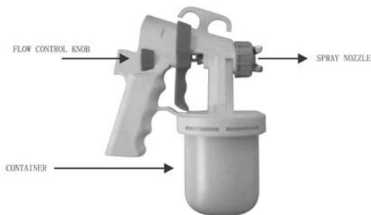
2) **The Spray Nozzle;** adjusts the fan spray pattern of the solution. It should be set to spray either horizontal (A) or vertical (B). To change the spray pattern, slightly loosen the adjustment ring, turn nozzle to desired position and retighten ring.
